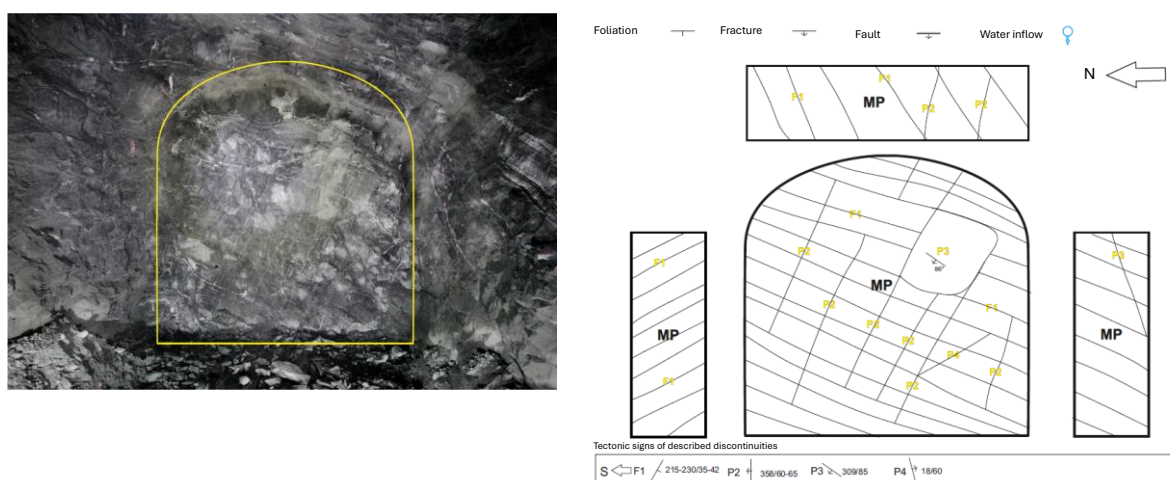
Fig. 23 – Example of the photo documentation and a drawing of the mine face in the geological documentation
