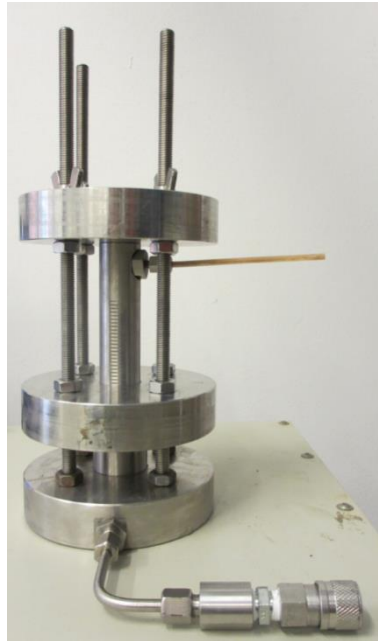
Fig. 10 Permeability chamber showing the coupling at the sample inlet for connection to the pressurising system
