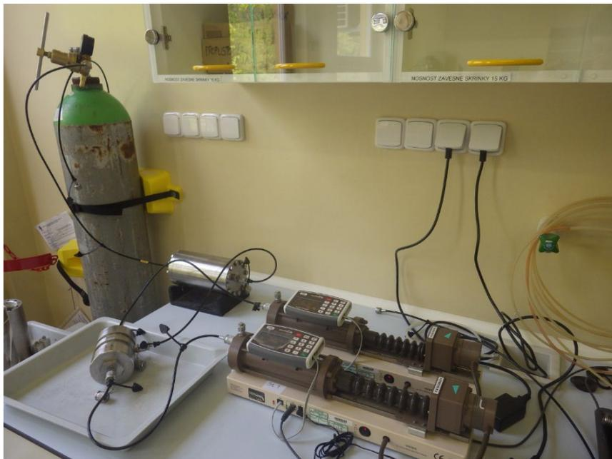
Fig. 6: Apparatus for the determination of the filtration coefficient  $K_f$  at the ÚJV laboratory.
