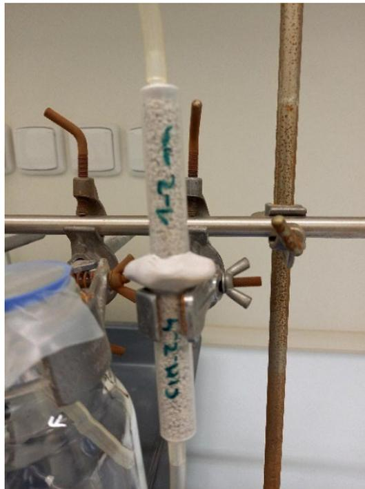
Fig. 9: Small column with the crushed cementitious material
