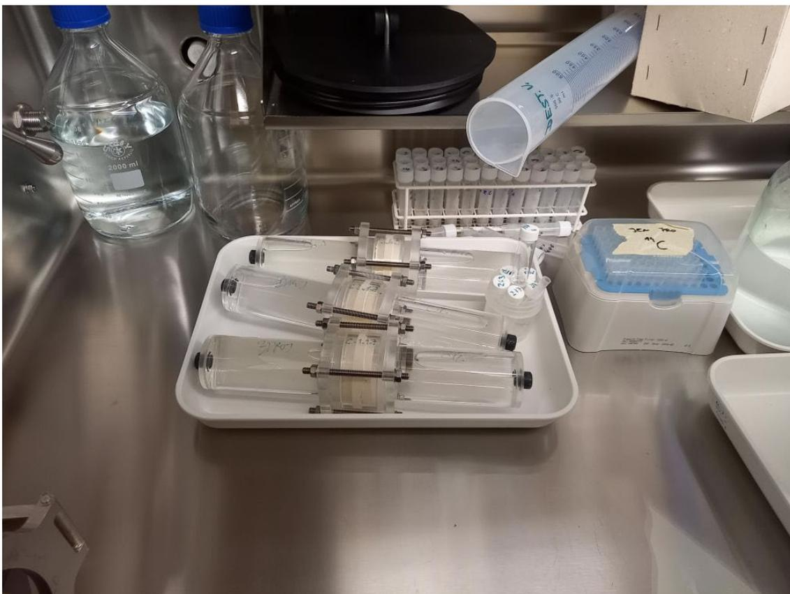
Fig. 11: Diffusion experiment performed in an inert atmosphere in the anaerobic glovebox
