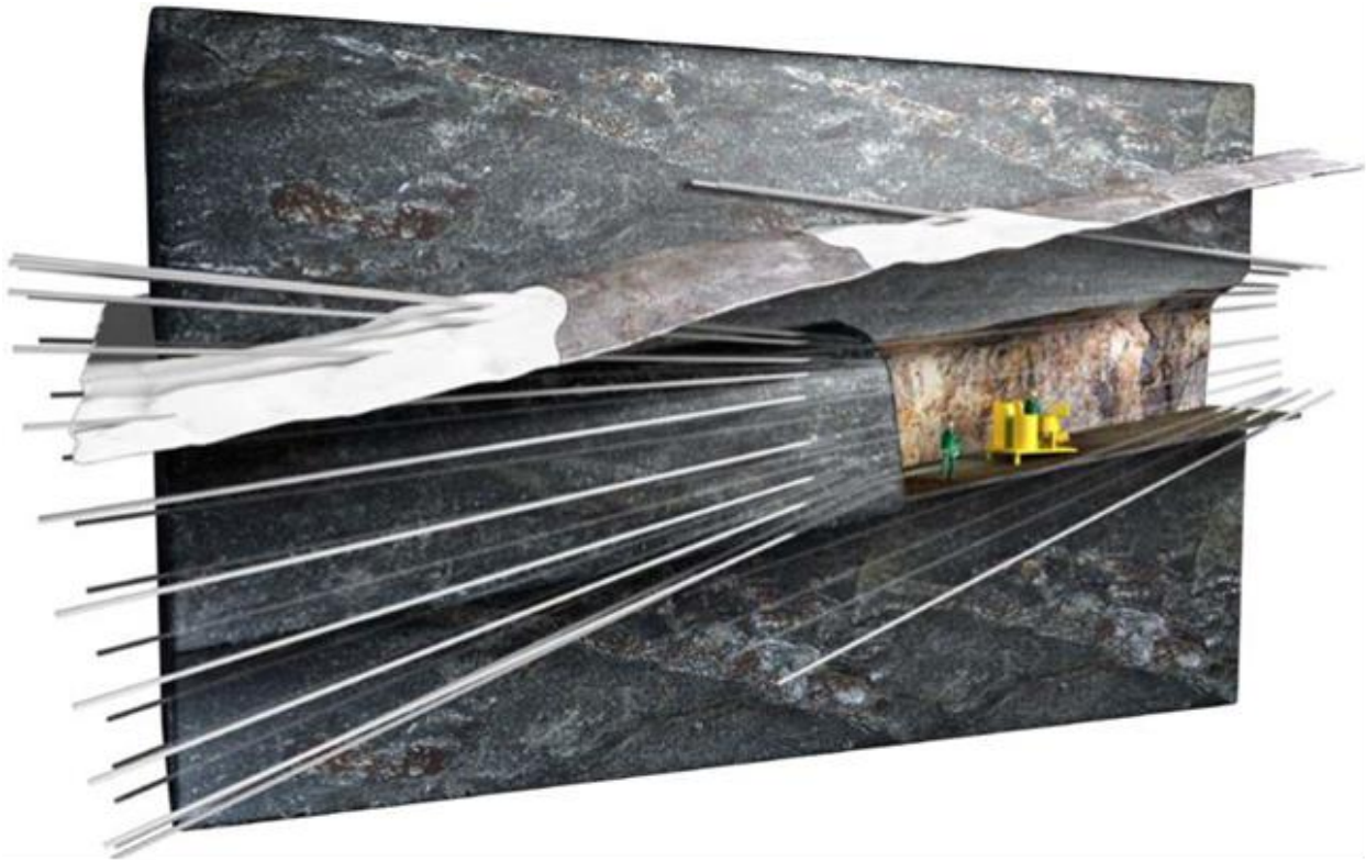
Figure 3-8. If pre grouting is neglected for technical or other reasons, the seepage water can remain too big, water chemistry can be totally changed and the risk that site will be spoiled as unsuitable for disposal grows. Figure SKB-report R-08-116 (SKB 2009).
