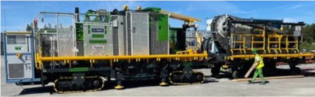
Figure 3-6. Posiva final vertical deposition hole boring machine for operating phase was completed in 2022 (Figure Posiva). This was developed according to experiences gained when boring numerous deposition holes in ONKALO with earlier prototype machine.
