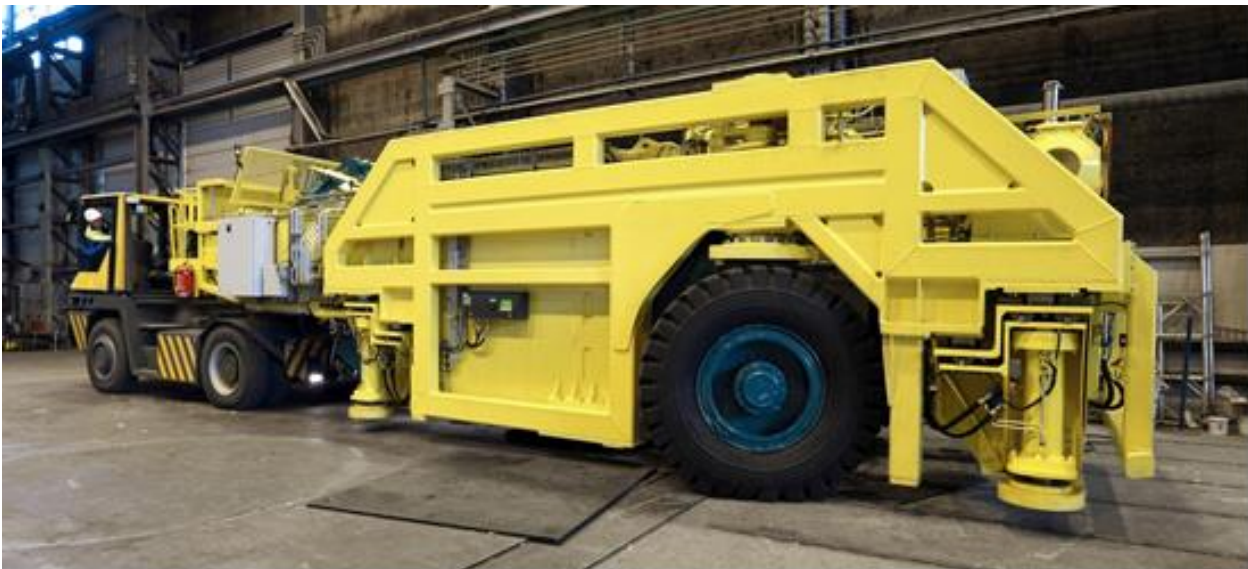
Figure 5-7. Posiva prototype canister transfer and installation vehicle (Figure Posiva). The assembly of the final version for operating is underway.
