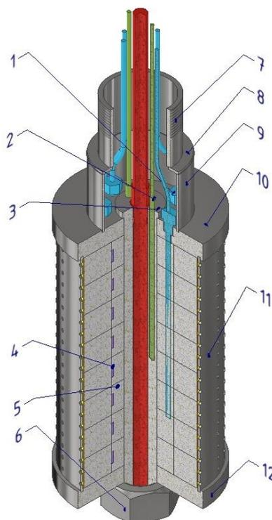
*Fig. 4 Design of the module for the corrosion tests at the Bukov URF. 1 – monitoring temperature sensors, 2 – managing temperature sensors, 3 – heating cartridge tube, 4 – corrosion samples, 5 – bentonite segments, 6 – M33 nut, 7 – G2" welding nipple, 8 – connecting plate, 9 – connecting tube, 10 – cover, 11 – perforated metal sheet with coarse and fine stainless-steel fabric, 12 – bottom*
